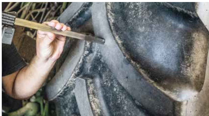
Figure 3: Wear measurement with depth stop
